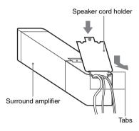
**3** Secure the speaker cord holder with the supplied screw (small).
